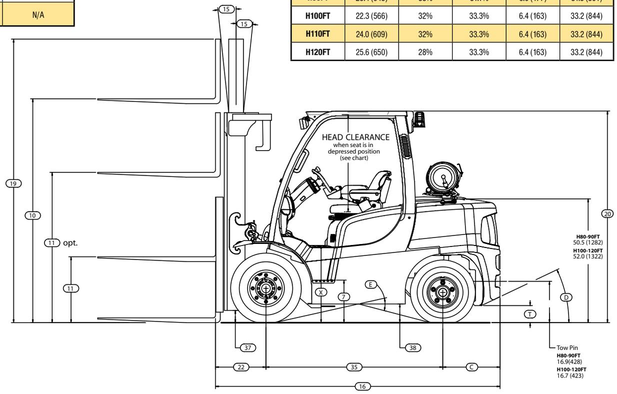
Circled dimensions correspond to the line numbers on the tabulated chart inside the Technical Guide. Dimensions are in inches (millimeters).
